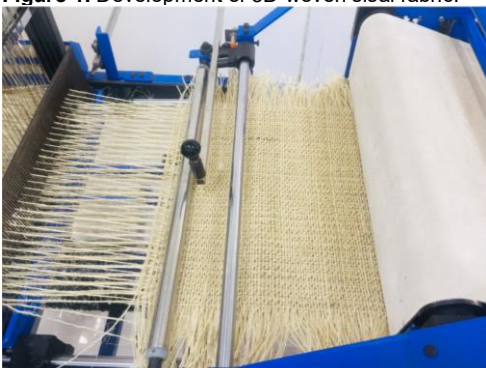
Figure 2. Development of 3D woven sisal fabric.
