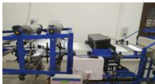
Figure 1 Customized weaving machine equipped with two beams and modified take-up system
